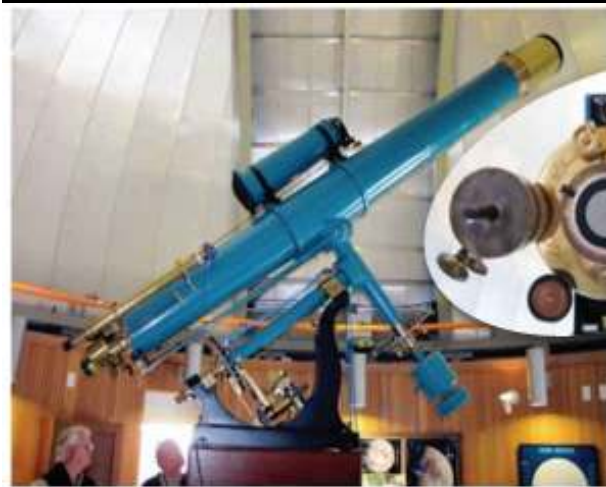
The Alvin Clark 8", f17 refractor named "Leah", showing the side view and "Business end". Note the large engravings on the brass endcap identifying it as an Alvin Clark telescope.
